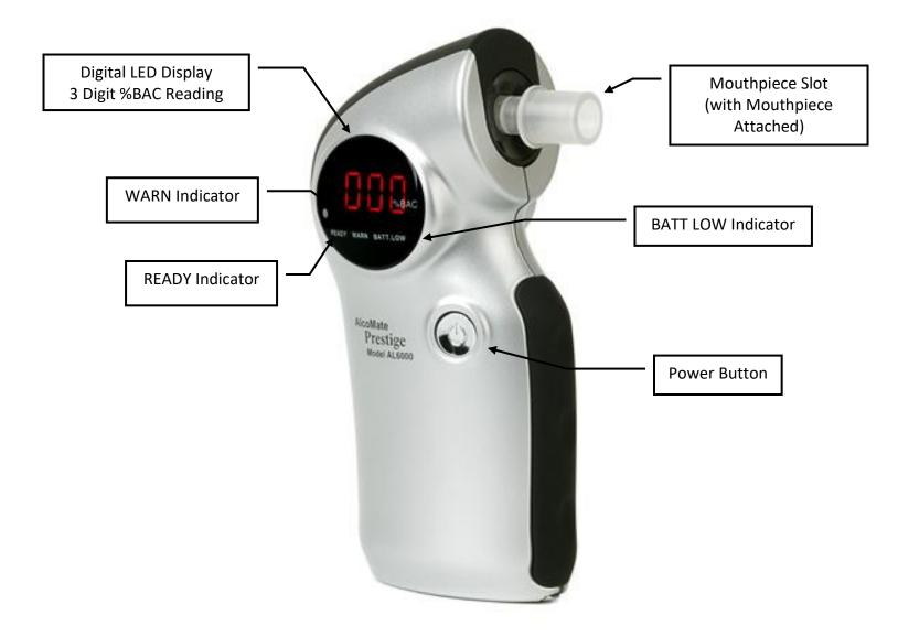
The AlcoMate Prestige AL6000 analyzes a breath sample to analyzes a breath sample to detect alcohol in the lungs. This reading is then converted to blood alcohol concentration (BAC). The AlcoMate Prestige uses an advanced oxide semiconductor sensor to detect alcohol. The Prestige is the original breathalyzer that features Pre-Calibrated Alcohol Sensor Modules to eliminate the need for recalibration. Just snap out, snap in and you're ready to go!
